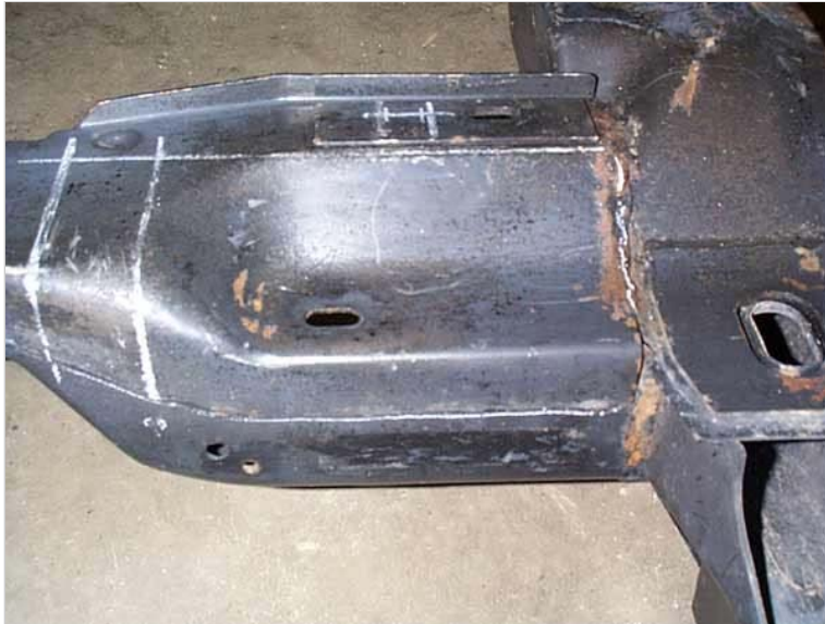
Cut & section cradle (before)
