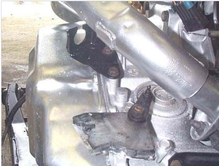
TH125 bracket cut off & welded to piece of 4T60 bracket
